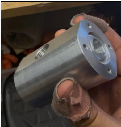
(Machined Components of Pyrotechnic Vent Valve Assembly) 6061 Aluminum
